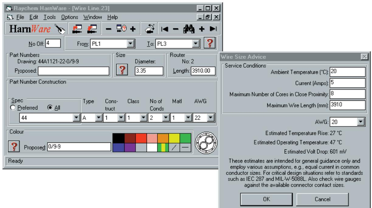
Fig. 4 Guidance on choosing wire type and wire gauge
